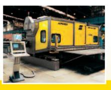
ALPHAREX is not only capable of cutting sheet material, but also of thick structural steel plates, stainless steel and aluminum.
