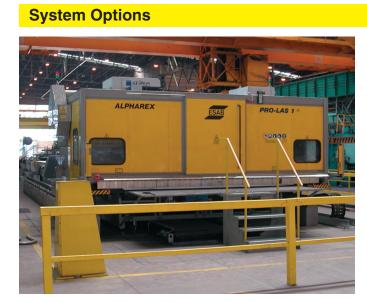
The PRO-LAS enclosure option provides Class 1 laser protection. It is optional on machines with a straight cutting head, but mandatory on machines with a bevel head.
