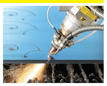
The optional laser bevel head allows fully automated variable bevel angle contour cutting from 0 to 45 degrees.
