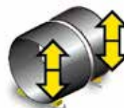
Joining of shell sections using roller beds with hydraulic fit-up system. Internal and external submerged-arc welding performed by a column and boom station.
