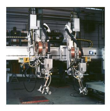
The combination of compressed air, flux feeding, automatic fill up of new flux and continuous recovery contributes to a welding station with less down time, cleaner working environment and high quality welds as a significant result.
