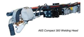
The Compact 300 is designed to weld with a maximum wire diameter of 4 mm, when welding carbon steel and a maximum wire diameter of 3.2 mm, for welding of stainless steel. The welding head is designed for single wire. The built-in pneumatic valve, to open or close the feeding of flux from the FFRS System (1), will be controlled from the PEK control box (2).
